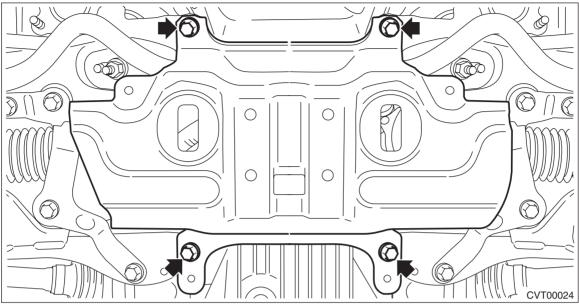
20) Install the center exhaust pipe. <Ref. to EX(H4DO(w/o HEV))-15, INSTALLATION, Center Exhaust Pipe.>
