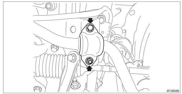
7) Remove the bolts which secure to the front housing, and separate the front arm and housing.
