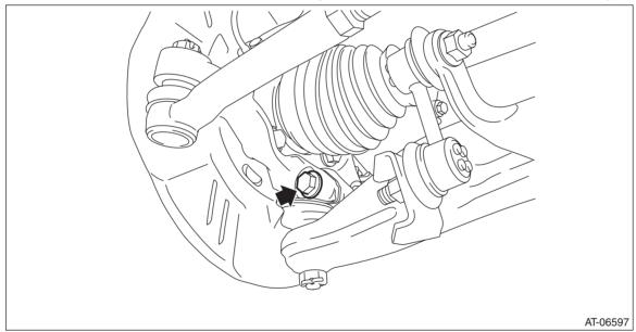
8) Using a crowbar, etc., pull out until the front drive shaft transmission side joint slides move smoothly. NOTE:
